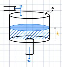
Here the output y is just the water level . We can now model the system as follows:
